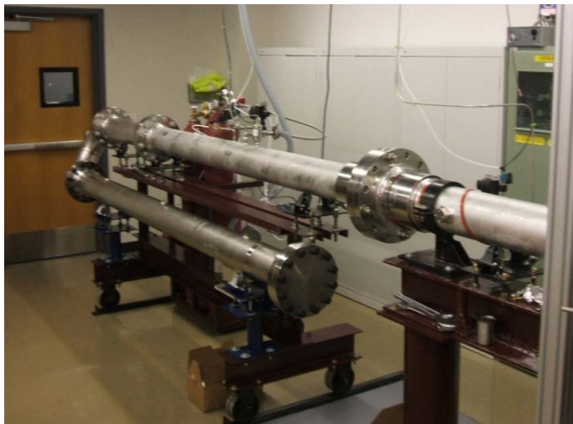
Kinetics Shock Tube 1 (30 atm)
