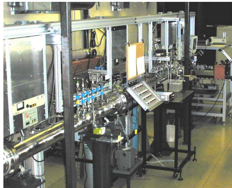
Kinetics Shock Tube 2 (30 atm)
