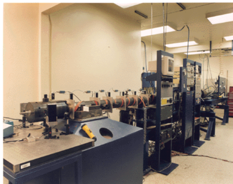
High Pressure Shock Tube (500 atm)
